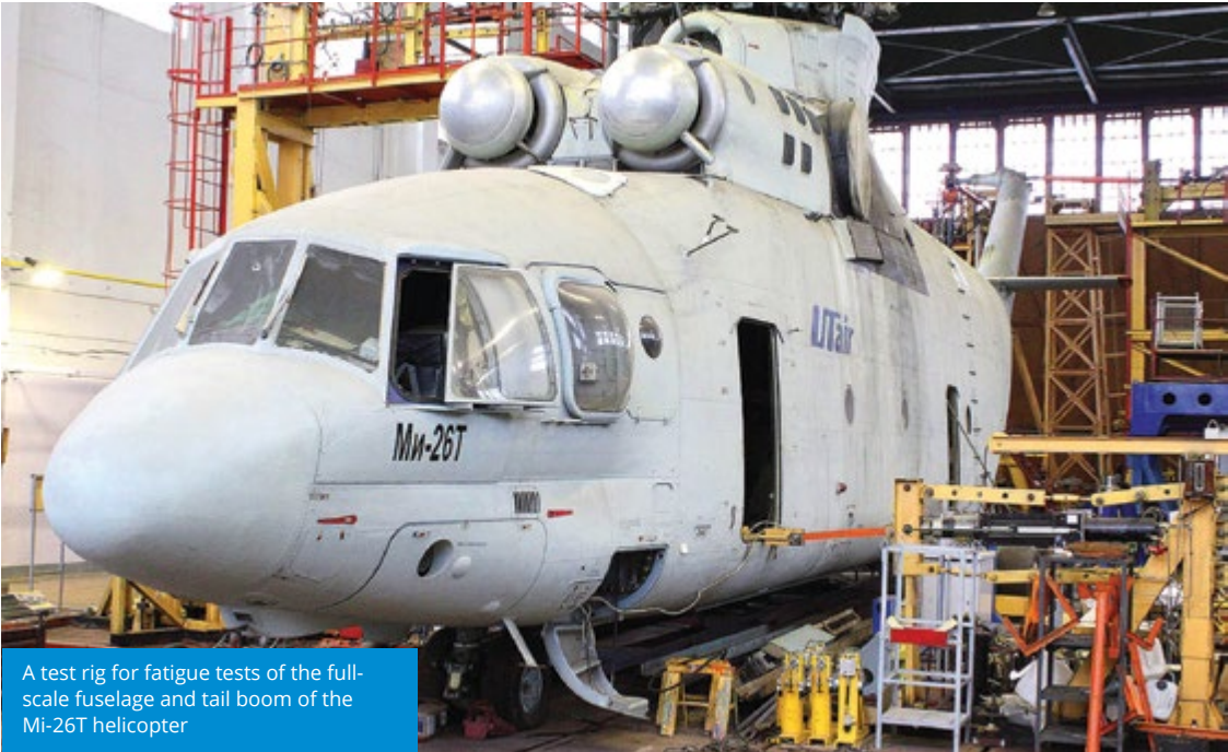
The arrangement of the test rigs for Mi-26T, Mi-38 and Ka-62 helicopters at the static testing shop of AVIATEST
