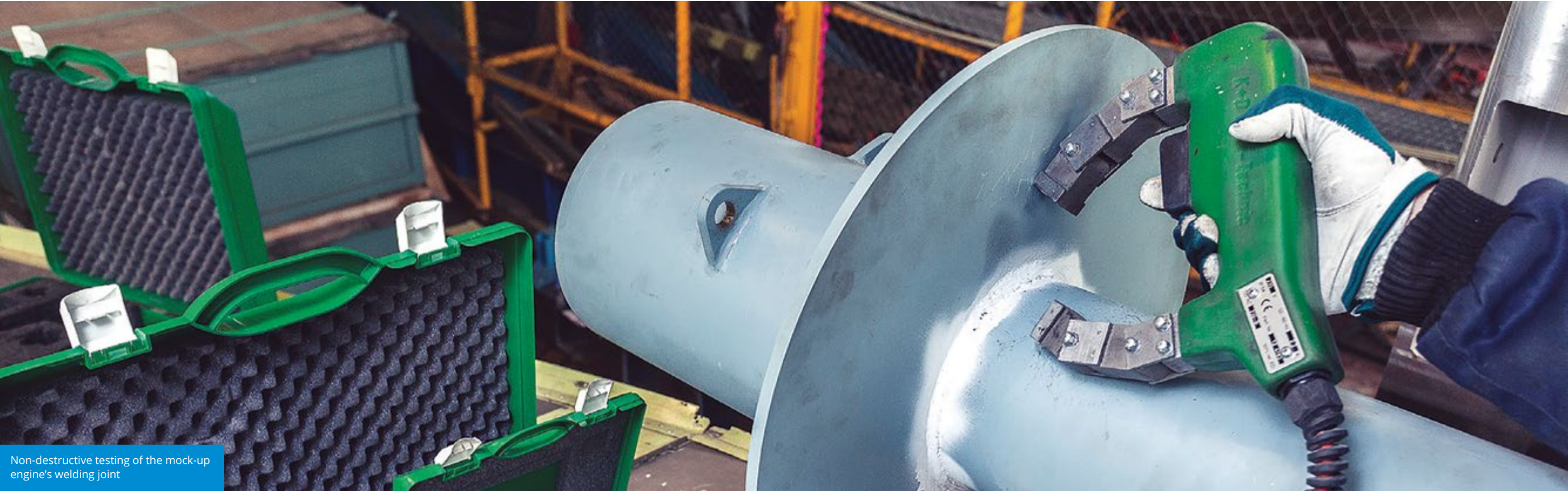
Eddy-current testing performed on one of the pressure bulkhead seals of the aircraft
