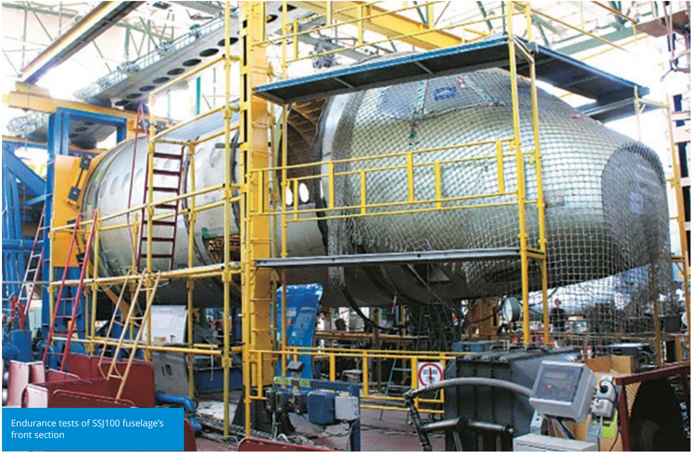
The arrangement of the fuselage sections of SSJ100 and MC-21 at the static testing shop of the AVIATEST laboratory
