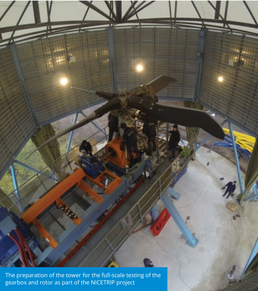
A test rig for testing gearboxes and transmissions of helicopters and their modifications
