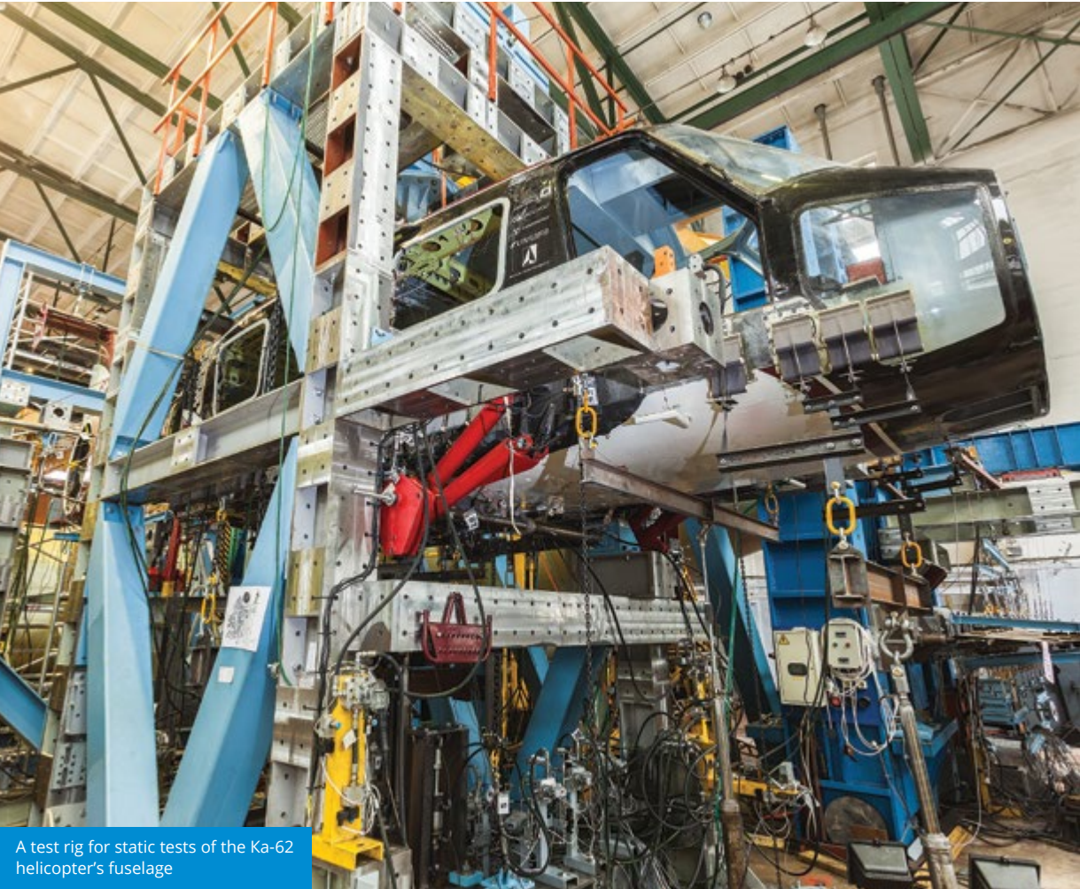
The arrangement of the test rigs for Mi-26T, Mi-38 and Ka-62 helicopters at the static testing shop of AVIATEST
